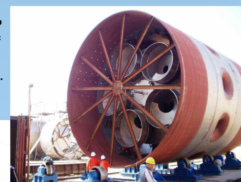
(Above) The ATP Center Support with Preheat Tube connections.
