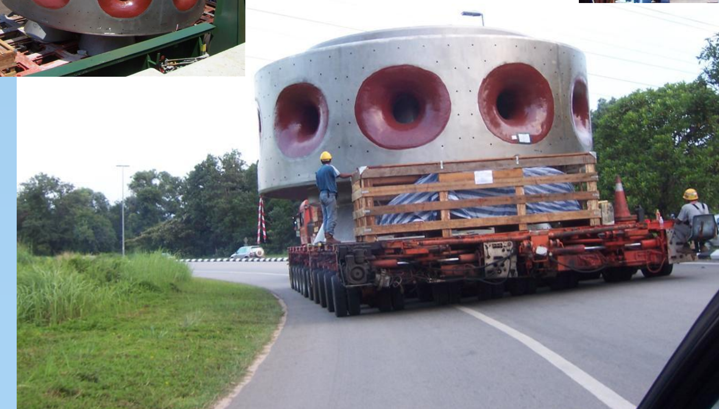
(Above) The ATP Center Support with Preheat Tube connections.
