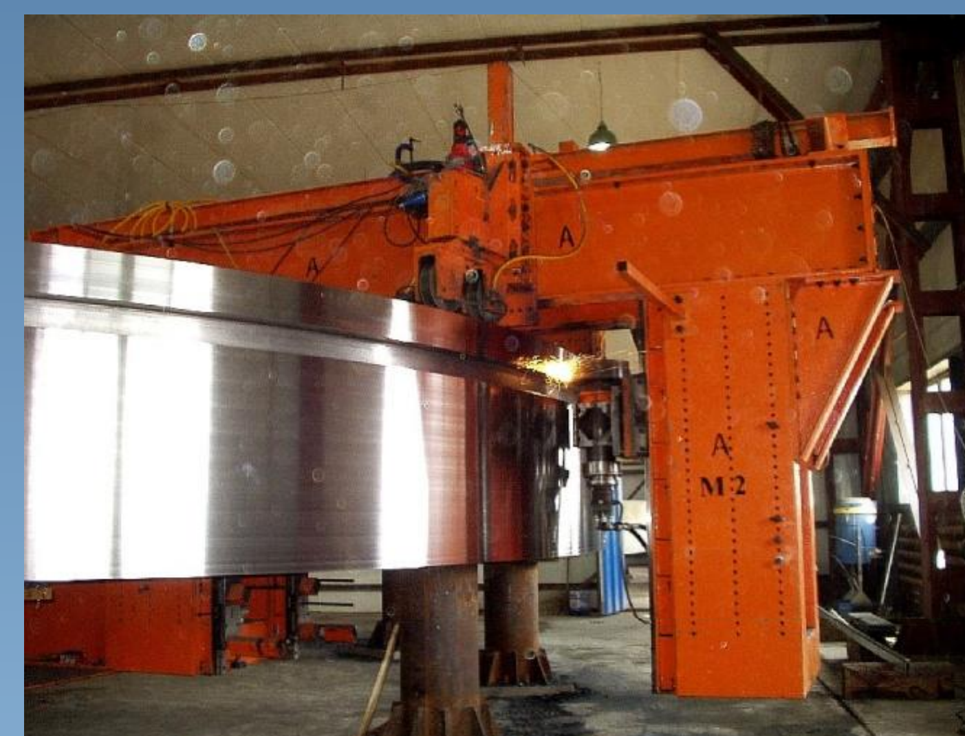
(Left) Field machining of the 11 m (36') diameter support tyres on-site. This was a leading edge field-machining operation successfully completed under challenging conditions in China.
